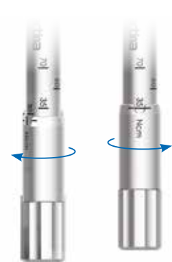
For decreasing the torque value, just turn the ring nut in an anticlockwise direction, until a value lower than the wanted one; then proceed with the screwing in a clockwise direction until the wanted torque value is reached.
